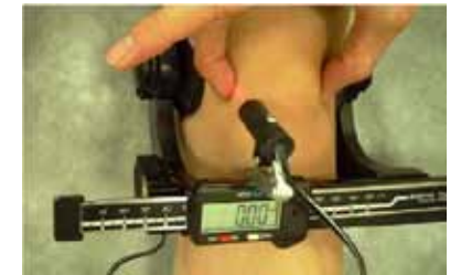
Figure 2. Initial position of the patellar mobility (set 0 mm of the digital caliper)
