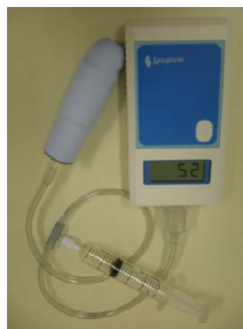
Figure 3. Perineometer (Peritron 9300V) Perineometry was performed by use of air-filled silicone sensor connected portable perineometer with a pressure transducer.
